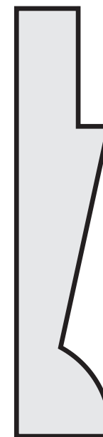
P133 3/4" X 3 1/8" RAISED PANEL MOULD
