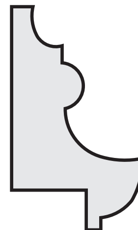
P128 1 3/8" X 2 5/16" RAISED PANEL MOULD
