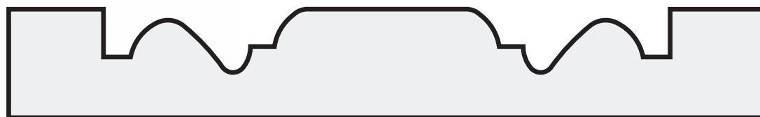
P153 13/16" X 5 5/8" CASING MOULD
